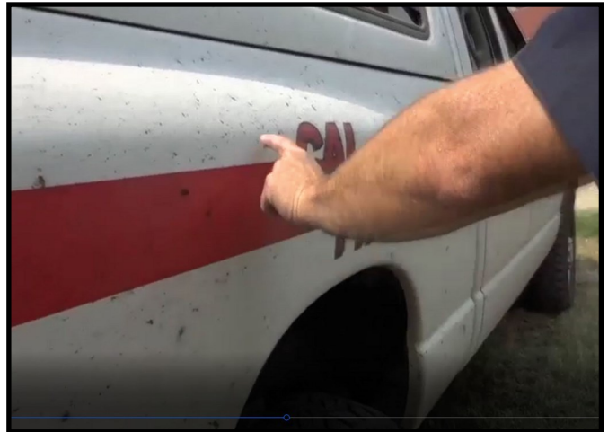
Fire Tornado Damage from Melted Asphalt
